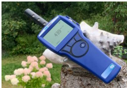
Figure 3: A handheld NDIR CO 2 measuring device calibrated with Keeling flasks. It shows a deviation of +10 ppm from the calibration source.
