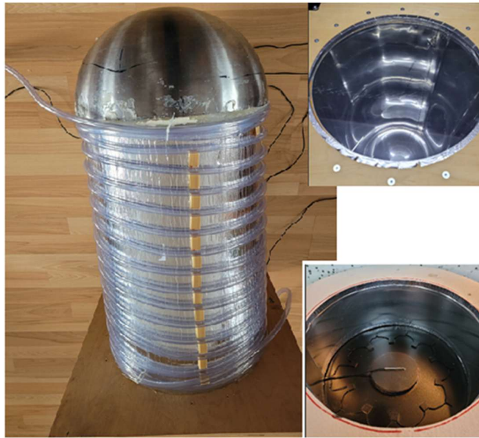
Fig. 2: Left: Gas cylinder with insulating wallpaper and PVC hose for heating with 51°C warm water, before the external thermal insulation was applied. Top right: View into the interior of the gas cylinder with the PE foil clamped between two wooden panels as the lower end. Bottom right: The blackened P_C plate beneath the gas cylinder with the thermal radiation sensors D_T and D_P , thermally insulated by a Styrofoam block with a mirrored aluminum inner wall.
