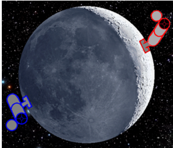
Figure 3. Simultaneous continuous functioning of the system of two SOTR-300VM depending on the change of lunar day and night for each telescope: at lunar nighttime – the telescopes system will continuously observe the Earth for more than 94% of the lunar day; at lunar daytime – the telescopes system will be continuously monitoring of the asteroid-comet hazard throughout the celestial sphere during 100% of the lunar day (Abdussamatov, 2024b).
